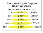
Beam Angle (50% max) 90 DEG 130 DEG Field Angle (10%) 20,000 lm Luminous Flux (IES) Light Efficacy (IES) >100 lm/W 27 UGR **Cutoff Classification** Cutoff
